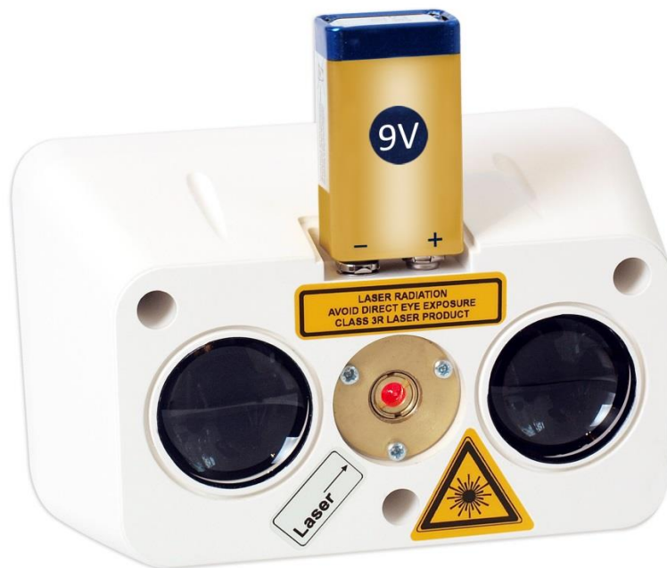
Fig. 2 DOP-6001R detector during optical path alignment
