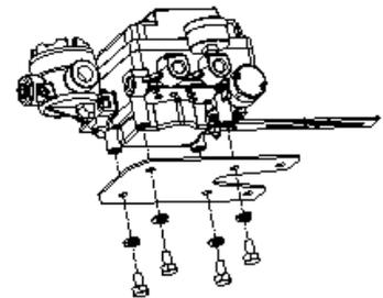
3. Attach the positioner with bracket to the actuator yoke – **DO NOT TIGHTEN POSITIONER COMPLETELY.**
