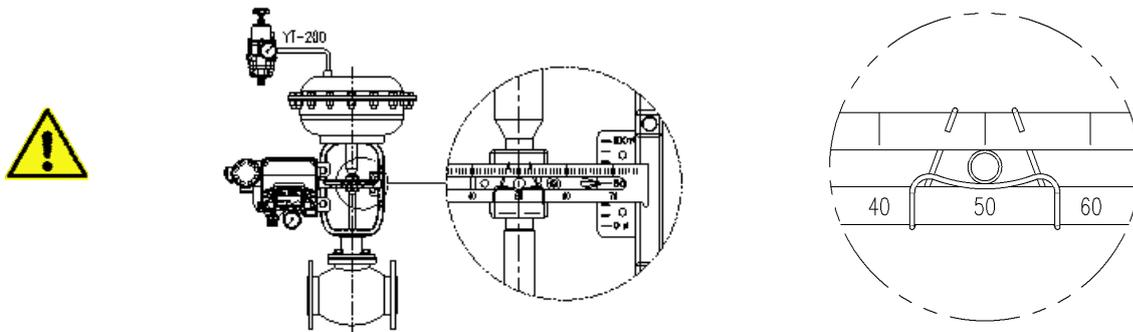
Proper way to connect feedback lever, connection pin, and lever spring
