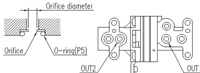
1. Remove the pilot relay assembly from the positioner.
