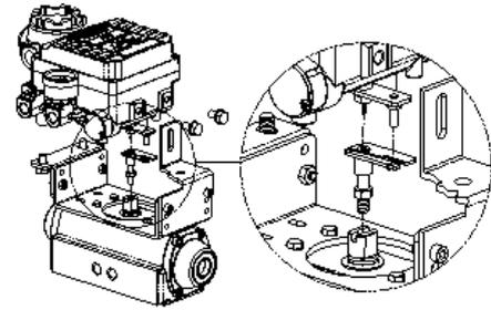
7. Tighten the positioner and the bracket with hexagon-headed bolts and plate washer **after checking the positioner's position.**
