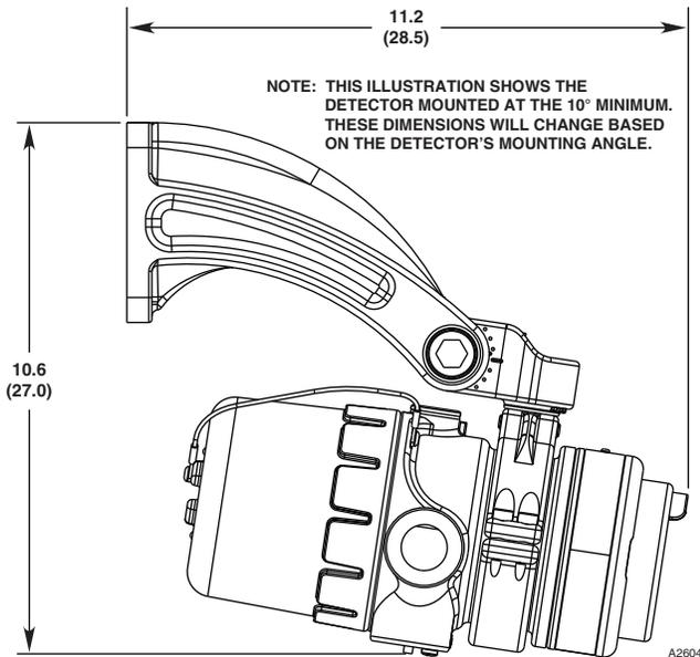
Figure 3— Q9033 Mounting Arm with Collar Attachment
