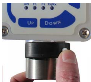
Fig. 2 From this position remove the magnet and the zero calibration procedure is terminated
