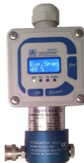
Fig. 2 From this position remove the magnet and the zero calibration procedure is terminated
