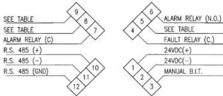
**Figure 8: Wiring Terminals**
