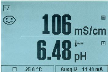
Measurement display with two primary values (above) and two secondary displays (below), i.e. 4 measured values can be simultaneously represented on the display
