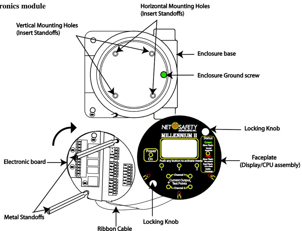
**Note:** To access enclosure grounding screw, remove the electronics module by following steps 1-7 above.
