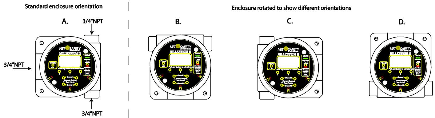
**Note:**The electronics module can be rotated to suit enclosure orientation.
