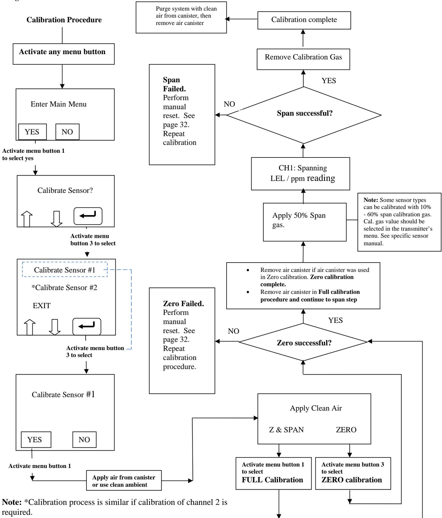
**Note:** \*Calibration process is similar if calibration of channel 2 is required.
