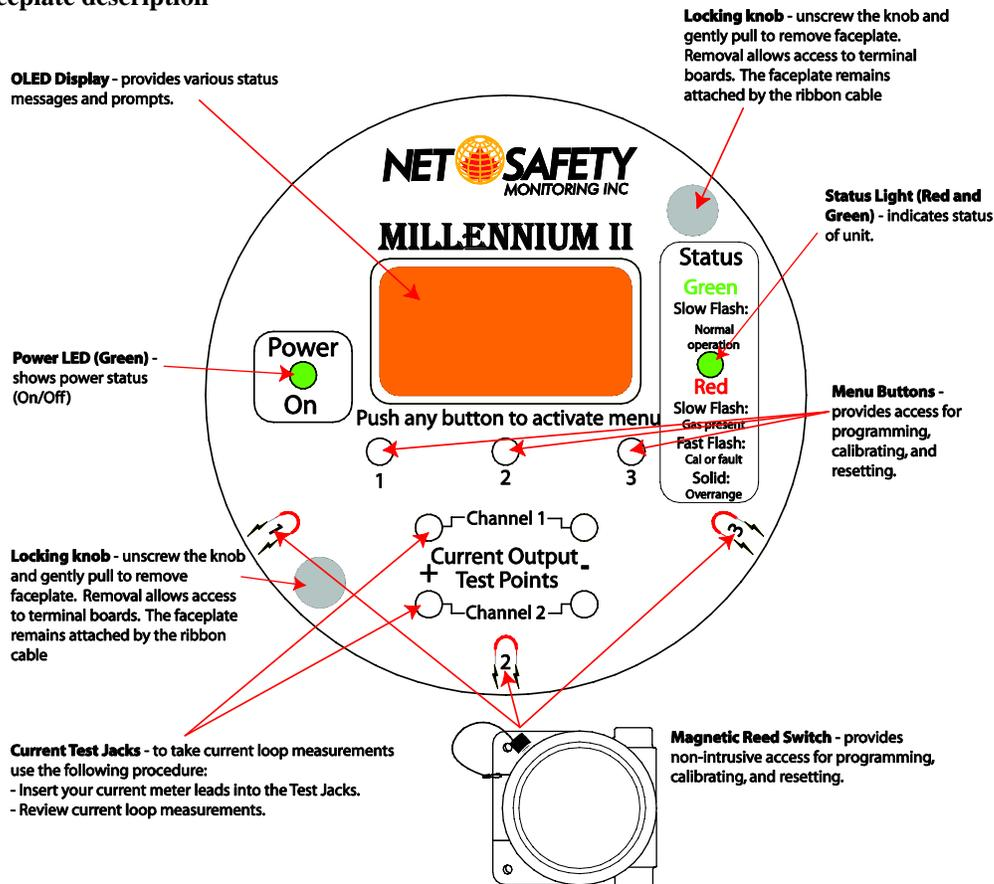
**Note:** A slow flash is defined as the Status LED being ‘ON’ for 50 milli-seconds and ‘OFF’ for 1 second, while a fast flash is the LED being ‘ON’ for 250 milli-seconds and ‘OFF’ for 250 milli-seconds and a very fast flash is the LED ‘ON’ for 50 milli-seconds and ‘OFF’ for 50 milli-seconds.
